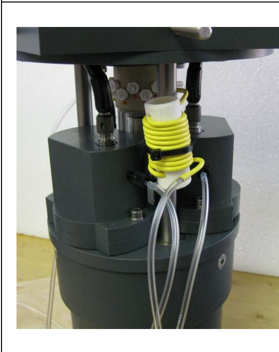
3. Install the cadmium column (if running nitrate)
