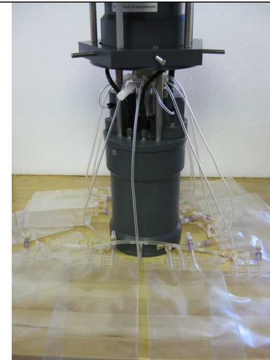
4. Lay-out the (filled) reagent bags and connect their supply tubes to the appropriate ports
