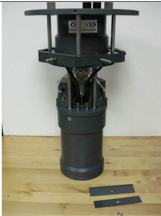
2. Remove the bag clamps from the pentagon shaped bag frame
