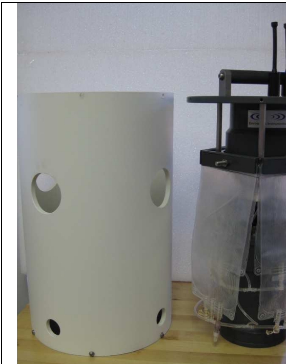
1. Remove the analyzer from the reagent housing / guard
